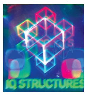
This holographic metode is possible to use for security purposes as level 1 or 2 security feature and for true color display holography as well. It is based at the fusion of three separate reference waves R, G, B, which illuminates the hologram from different angles. By special calculation we can generate microstructure of the embossed hologram witch behaves as a volume hologram. It means that colors are stable for wide range of angle of view in horisontall and vericall parallax.
